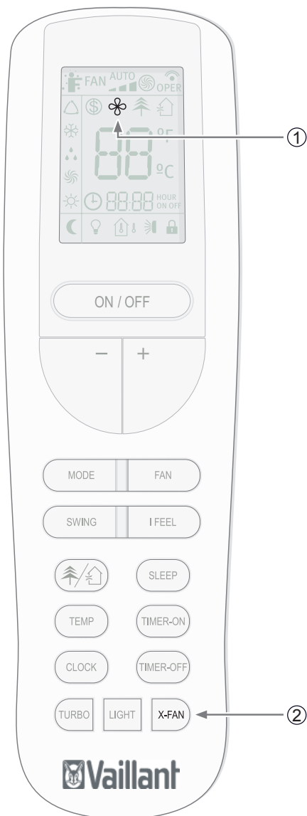
Fig. 7.19 X-FAN function selection.
