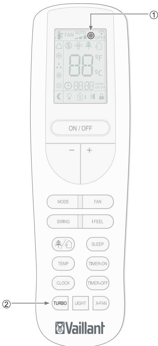
Fig. 7.18 TURBO function selection.
